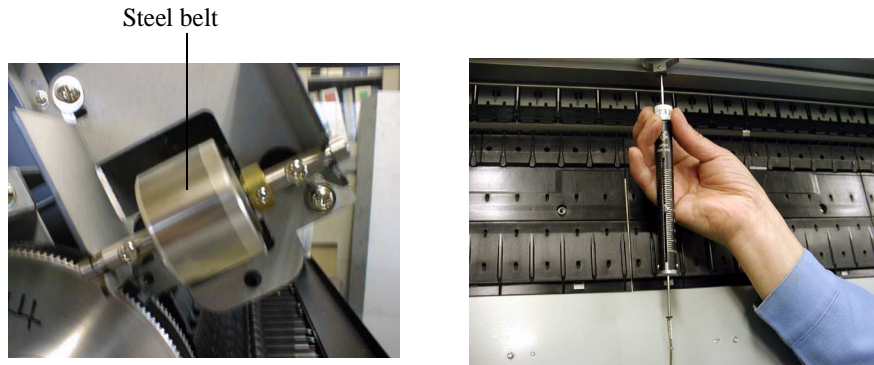
Figure 5-2. CR steel belt tension adjustment
